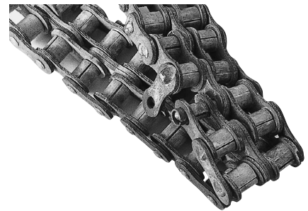
Fig. 31 Corrosion of stainless steel roller chain
